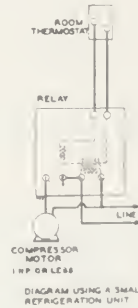
25-46. Wiring diagram of thermostat, relay combination for small comfort cooling units. (White-Rodgers Electric Co.)
